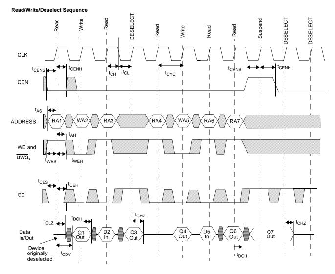
The combination of  $\overline{\text{WE}}$  and  $\overline{\text{BWS}}_x$  (x = a, b, c, d) to define a Write cycle (see Write Cycle Description table).  $\overline{\text{CE}}$  is the combination of  $\overline{\text{CE}}_1$ ,  $\text{CE}_2$ , and  $\overline{\text{CE}}_3$ . All chip selects need to be active in order to select the device. Any chip select can deselect the device. RAx stands for Read Address X, WA stands for Write Address X, Dx stands for Data-in X, Qx stands for Data-out X.
